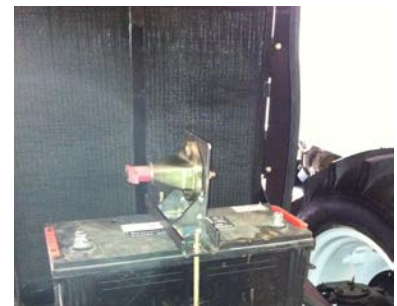
Fig. 3-26 Main power switch
