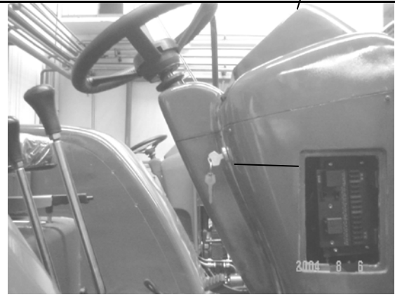
Fig. 3-78 Central electrical control box
