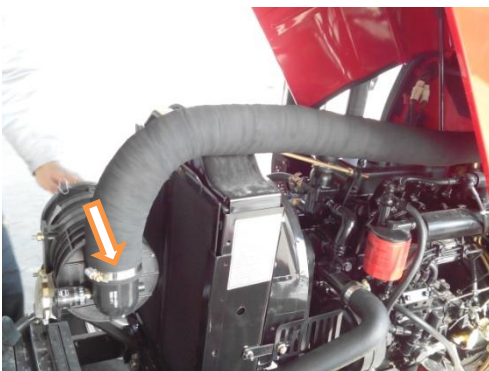
Dry-type air filter intake system clamp
